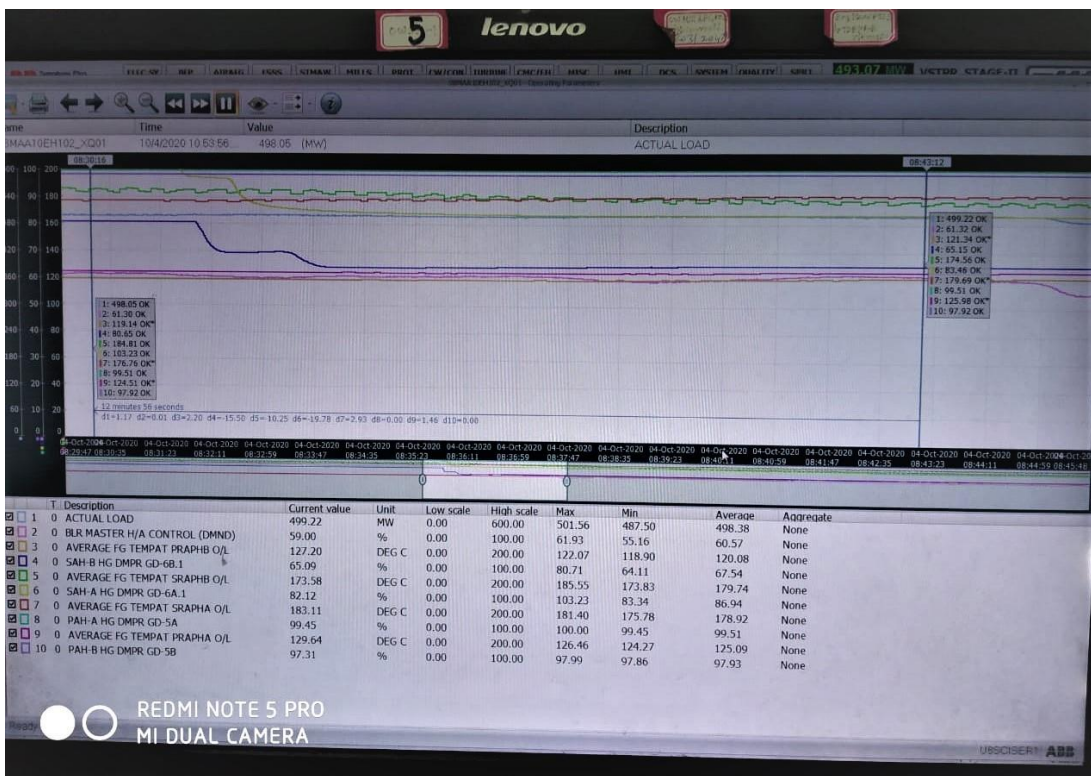
Fig 13. Trend of Flue Gas Outlet Temperature post throttling
