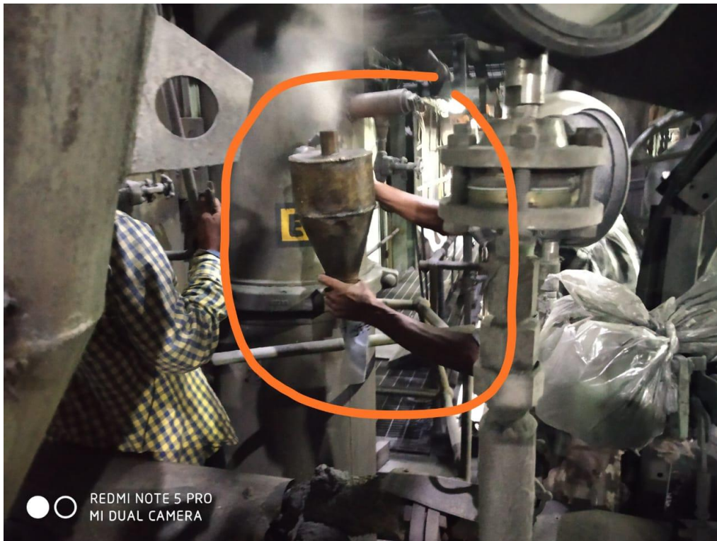
Fig 5. Corner wise coal fineness sample collection in progress using cyclone separator .
